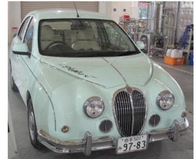
Test vehicle equipped with an engine hood made of fiber reinforced composites (modified lignin) Photo provided by Miyagi Kasei and AIST Partner; MITSUOKA MOTOR
